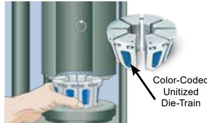
Lubricate die bowl using a premium quality lithium-base grease. Place unitized die-train into the adapter bowl. Select die and die ring by hose size and type. See decal on crimper for proper die set. **Note:** Die sets have color-coded cavities indicating size and have the fitting series and dash size stamped on the top.
