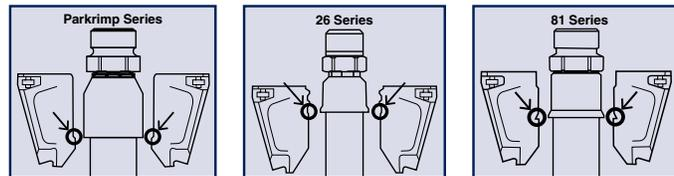
Position the hose and fitting in dies from below. Rest bottom of coupling on die step using the PARKALIGN® feature.
