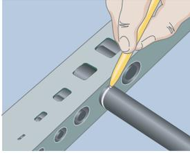
Mark the hose insertion depth and push hose into fitting until the mark on the hose is even with the end of the shell. Lubricate hose if necessary, however, **DO NOT lubricate if using spiral hose.** See Hose Insertion Depth table on previous page.
