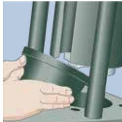
Lubricate die bowl using a premium quality lithium-base grease. Carefully insert the adapter bowl, 83C-OCB, into the base bowl. The adapter bowl must be tilted toward the back of the crimper during insertion.
