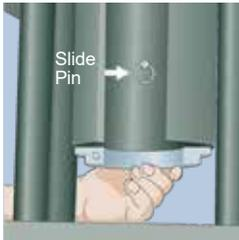
With the pusher in the full up position, lift the back half of the split die ring. Lock it in the up position by pushing the slide pin in. (The slide pin is located inside the pusher at the back.)
