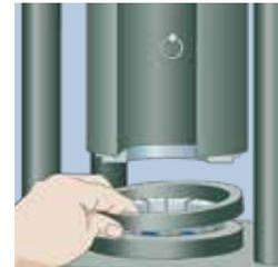
If required, place spacer ring on locating step of adapter bowl. Reference decal on crimper for tool selection.
