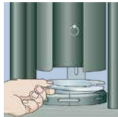
Insert the front half of the split die ring aligning the pins in the back half with the hole in the front half.
