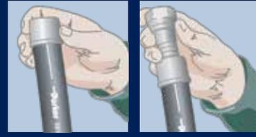
Place 81 Series Shell onto end of hose and make sure the end of the shell lines up with the Insertion Depth mark.
