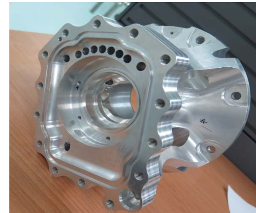
MANIFOLD ASSEMBLY SHUTOFF VALVE/ (Al Alloy, B737)
