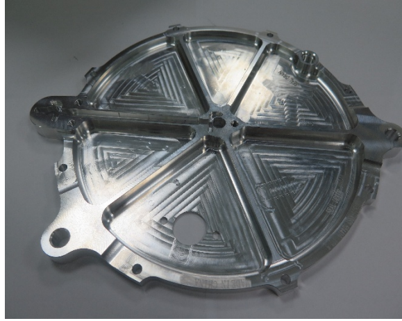
Cover Assembly, System 1&2, (Al Alloy, Cseries)
